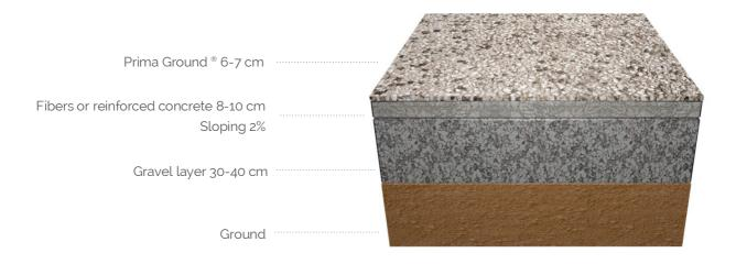
Prima Ground® On a sloping waterproof concrete base Version for traffic
