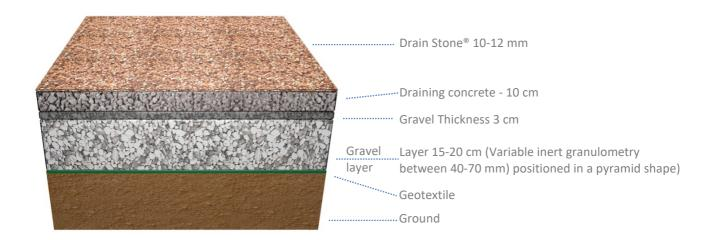
Prima Drain Stone® on a permeable concrete base - Traffic version (≤ 3,5 ton)
